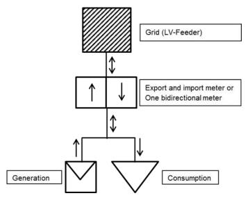
Figure 1: Proposed Metering Arrangement
